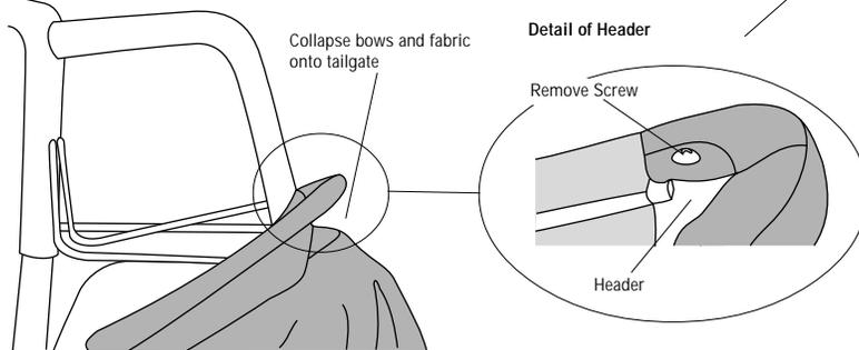
**Manufacturing Note:** Due to a recent header assembly modification by Daimler Chrysler, the plastic strip on the windshield header may have 8 screw locations instead of 14. Both attachment numbers of screws will securely fasten the header and perform as the original design was intended.
