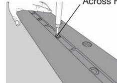
Slide Extrusion along the Front Edge of the Channel to remove Top
